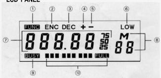
1 FUNCTION 2 CTCSS ENCODE 3 CTCSS DECODE (option) 6 OFFSET SHIFTI DIRECTION + @ OFFSET SHIFT DIRECTION -@LOW POWER MODE 7 FREQ/CHANNEL DISPLAY  MEMORY CHANNEL NO. (WHEN FREQ. IS DISPLAYED AT (7)) "FL" WHEN FREQ. LOCK IS ON. "P" WHEN PRIORITY SCAN IS ON.
