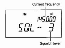
The squelch level increases when the dial is rotated clockwise, and decreases when the dial is rotated counterclockwise.
