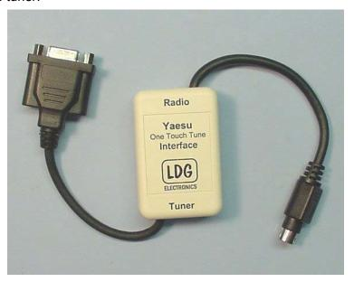
**Important!** Before making any connections, be sure that the DC power to the radio has been turned off. The radio does not fuse the DC power to the tuner and internal damage to the radio could occur if the Y-OTT power connector conductor comes in contact with ground. Always remove DC power from the radio prior to making any connections with the Y-OTT.
