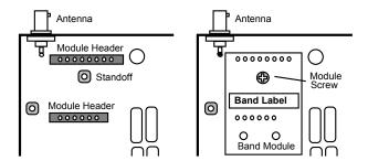
The band-module headers are located directly below the BNC antenna connector. Line up the module and install it component-side down, as shown. Fasten in place using the module retention screw and reinstall the case. *Note that the retention screw should always be used to ensure firm seating and good grounding.* Also, note that a filter module must be installed for the DDS to recognize a band of operation.
