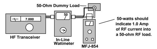
Set the meter's *Range* selector to 1-A. For meaningful results, *your wattmeter must be accurate and the 50-ohm load free of significant reactance*. To test, apply a 50-watt CW signal to the load. You should observe a full-scale reading of 1.0-A (100 on the scale). If results vary significantly from this reading, adjust trimpot R3 for the correct indication. Trimpot R3 is located on the unit's pc board below the sense coil.
