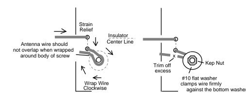
**Halyard Support:** The antenna may be center-supported using halyard mounting holes provided in the feed block. Connect as shown:
