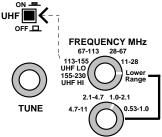
1. LF, HF and VHF Operation: The Lower Range rotary switch selects four LF and HF bands (0.53-11.0 MHz). The Upper Range switch selects 5 HF and VHF bands for 11-230 MHz coverage. Note that the Upper Range switch must be set *fully clockwise* to the Lower Range position for the lower-range band selector to function. The variable Tune control (VFO capacitor) provides a small overlap at each band edge to ensure gap-free tuning across the spectrum.
