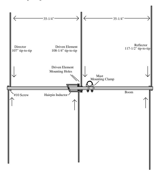
[ ] Find two (2) 59-1/4" reflector element sections and repeat the same mounting procedure at the back end of the antenna.
