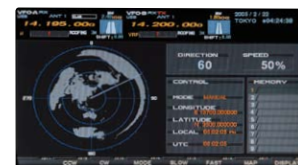
■ Antenna Bearing Indication using Great Circle Map
