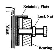
Grooves for installing guy attachment fitting allow easy tightening.
