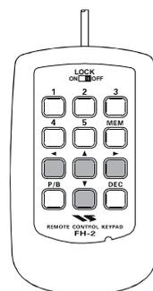
4. Press the **FH-2**'s **[1] ~ [5]** key to select the desired Message Memory Register into which you wish to program the text.
