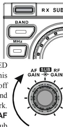
6. Press the **[BAND]** button corresponding to the Amateur band on which you wish to begin operation.
