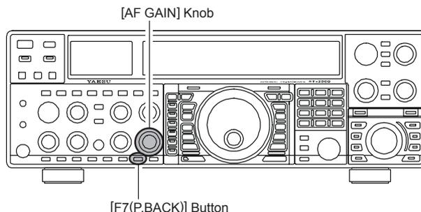
Pressing the **[F7(P.BACK)]** button once more will halt the recording, and the “**REC**” icon will go out.
