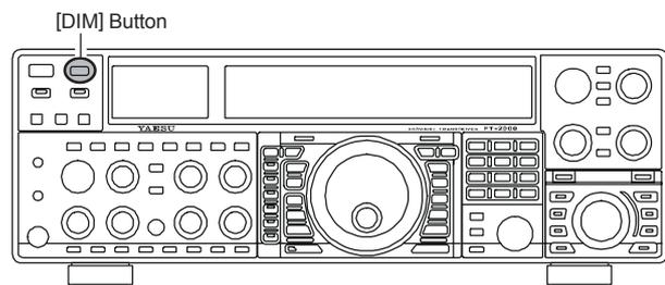
You may also customize the amount of brightness reduction engaged by the pressing of the **[DIM]** button, and may use different brightness levels for different front panel areas. Menu item “**008 diSP DIM MTR**” adjusts the brightness level of the analog meter; while menu item “**009 diSP DIM VFD**” sets the brightness levels of the frequency display (these settings are effective only when the **[DIM]** button is pressed).
