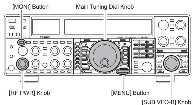
9. When you have completed all adjustments, press and hold in the **[MENU]** button for two seconds to save the new settings and exit to normal operation. If you only press the **[MENU]** button momentarily to exit, any changes you performed will not be stored.
