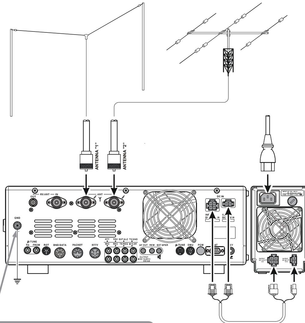
Use a short, thick, braided cable to connect your station equipment to the buried ground rod (or alternative earth ground system).
