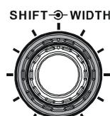
Referring to Figure B, you can see the default bandwidth with the [WIDTH] knob set to the 12 o'clock position.
