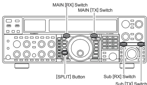
During Split operation, the Main (VFO-A) register will be used for reception, while the Sub (VFO-B) register will be used for transmission. If you press the **[SPLIT]** button once more, Split operation will be cancelled.
