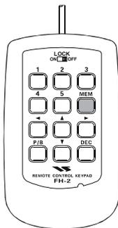
3. Press any of the **FH-2**'s keys numbered **[1]** through **[5]** to select that memory storage register. If you do not press the **PTT** key (see next step) within five seconds, the memory storage process will be cancelled.
